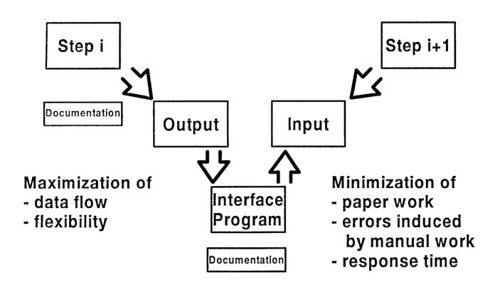
Fig.3 Element of process chain
