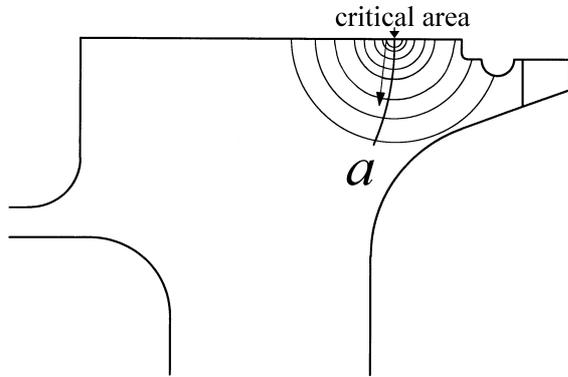
**Figure 2:** Analysed crack fronts and crack path  $a$
