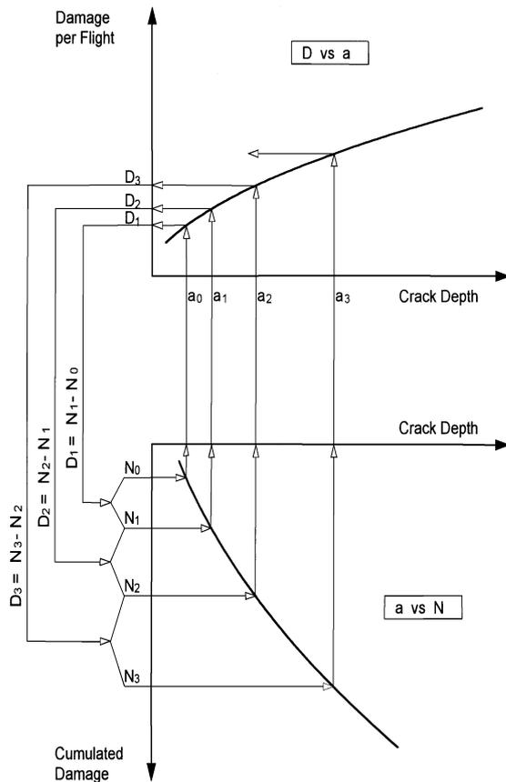
**Figure 6:** Procedure to simulate the damage accumulation
